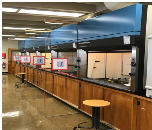
Figure 2. Fumehoods separation with Plexiglass panels
